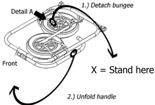
Stand on the nearside of the trailer so that the handle is nearest to you. Rest the trailer on it's trolley wheels and hold it upright by gripping the hinge or hand cuff with your left hand. We find it best to use this position for the whole folding sequence.
