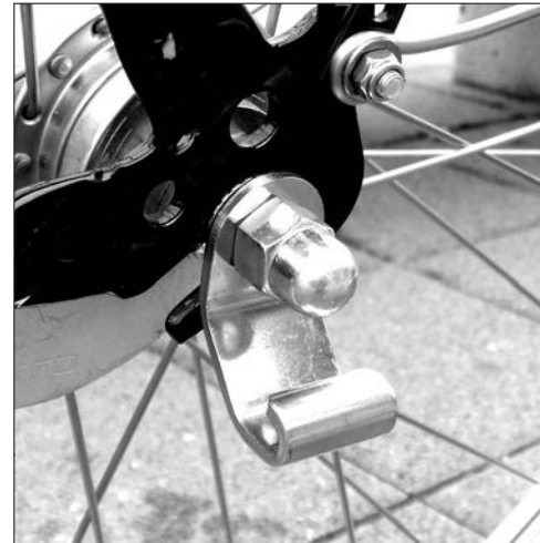
22. With nutted axles the bracket sits between essential washers and the nut
