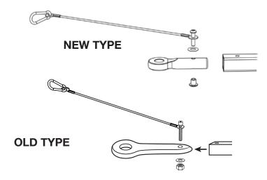
Older trailers are fitted using a bolt, washer and nyloc nut. New trailers are fitted using a bolt and a binding bolt on the other side. Check which parts you need. Both types are included.
